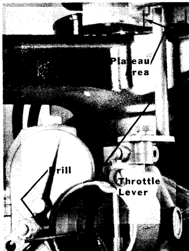
Figure 5. Checking Throttle Shutter Opening
