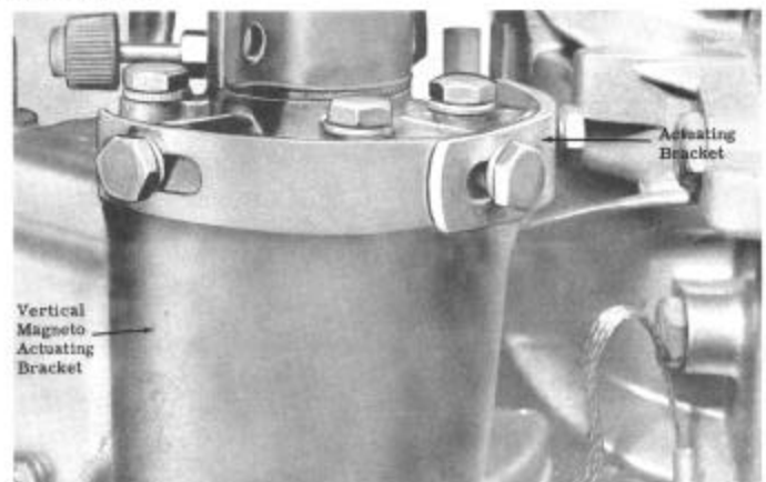
Figure 5. Adjusting Magneto Actuating Bracket
