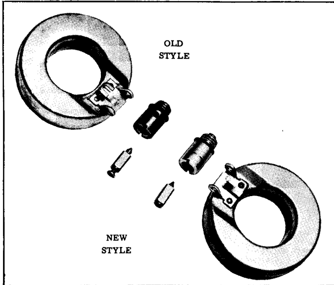
Figure 10. New Style Inlet Needle and Seat, Mark 20H C. Float Adjustment, Mark 55H
